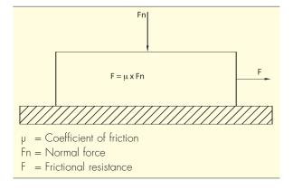
other types of friction, linear bearings fitted with balls or rollers offer not only much lower frictional resistance, but also an almost complete absence of static friction. For driven systems you have to take into account that the friction also includes the drive system that is chosen.
