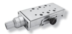
PM's lead screw tables series **RT-..-SRM** are miniature cross roller translation tables for manual operation. The tables provide accurate positioning capability and extremely smooth running operation along a linear axis. A positive position locking device eliminates drift when idle. RT-SRM slides are equipped with crossed roller ways achieving high load carry capacity and stiffness with very smooth motion.
