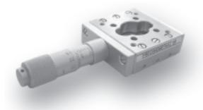
PM's positioning stages type **MT** are single-axis micrometer driven translation tables, designed for microscope-based inspection applications. Like all PM stages, MT stages are assemblied with crossed roller ways to assure unsurpassed travel performances in flatness and straightness and excellent stability.
