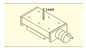
Inverted Load Capacity: is specified similar to normal load exept in an upward (tension) direction.
