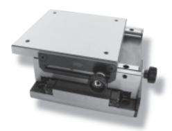
PM's XY-tables type **KT** are compact two axis crossed roller tables with equal strokes for manual operation. The tables are low profile designed and equipped with precision crossed ways. They can operate in every direction and locked in every position. For manual driven operation we supply model **KT-SRM** with a side mounted lead screw. Table and bearing specifications are similar to model KT.
