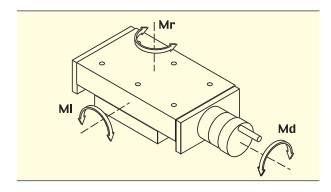
Maximum Speed: the highest speed recommended to prevent degradation of positioner life. For lead screw and ball screw driven tables, this may be calculated by multiplying the listed rps. (revolution per second) by the screw lead.
